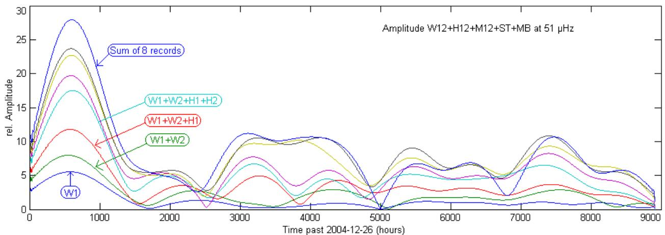
The measurement of the phase relationship is an indispensable tool to determine the direction to a vibration source. If the distances of all the receiver stations from the transmitter are identical, all received oscillations are *in phase*. Conversely, the following applies: If the recorded oscillations are *in phase*, the distance between source and all gravimeters is equal.
