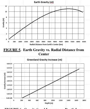
FIGURE 6. Gravitational Increase vs. Depth from Greenland Borehole Measurements
