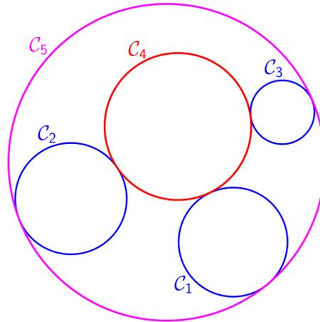
Figure 1: The Problem of Apollonius: *“Given three coplanar circles (e.g.  $C_1$ ,  $C_2$ , and  $C_3$ ), construct the circles that are tangent to all three of them, simultaneously.”* There are eight solution circles, two of which ( $C_4$  and  $C_5$ ) are shown here.
