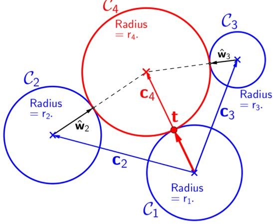
Figure 2: Definition of variables used for identifying the solution circle  $\mathcal{C}_4$ .
