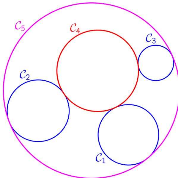
The Problem of Apollonius: *Given three coplanar circles, construct the circles that are tangent to all three of them, simultaneously.*
