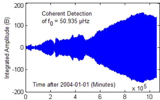
It can be seen that the mysterious vibration near 50.935  $\mu\text{Hz}$  has obviously been fueled twice: in March 2004 by a weak earthquake and in December 2004 by a much stronger one. Because of the better SNR, only the latter is examined.
