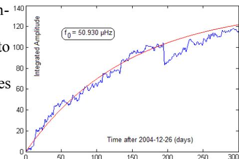
Now, for comparison and using the same program, the original data series of station H1 is replaced by a synthetic attenuated oscillation ( $f_0 = 50.935 \mu\text{Hz}$ ). The initial amplitude and the damping are varied until exactly the same output signal of the integrating detector is obtained. This synthetic oscillation is described by
