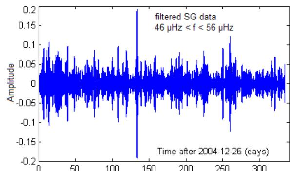
The damping of this mysterious oscillation on  $f_0 = 50.935 \mu\text{Hz}$  may be characterized by the very high Q-factor  $Q = \pi f T_0 = 3346$ . Perhaps it is one of the long-sought Slichter triplet lines.
