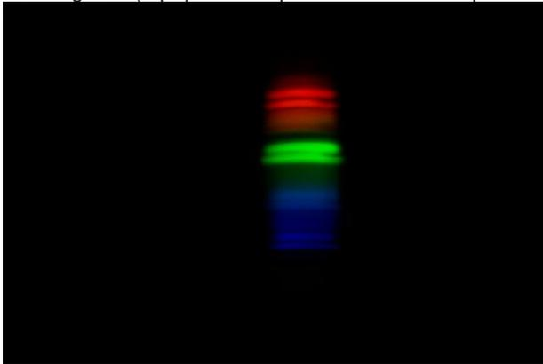
The amplitude of the wave increases the more the paper slit's angle decreases to the spectroscopy slit. When the paper slit is parallel to the spectroscopy slit, all emission lines have a line going through them. A larger angle to the spectroscopy slit will produce a more squished spectral wave, until 90 degrees is reached, when the spectral wave straightens out into one continuous line.
