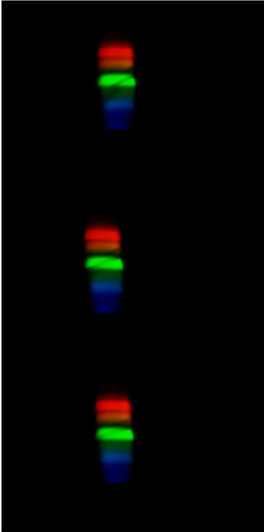
This phenomenon also occurs with a continuous spectrum source, but without the wave pattern. The shadow from the paper slit on the spectrum rotates almost 90 degrees and is always a straight line.
