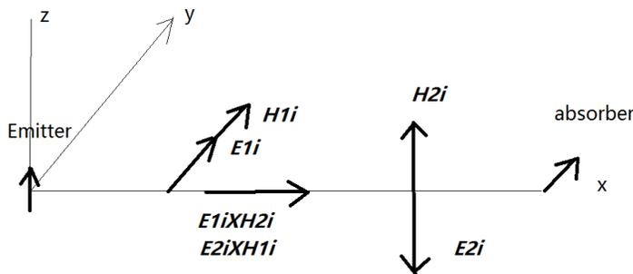
Figure 6. The current of the emitter is perpendicular to the current of the absorber. The filed of  $\mathbf{E}_{1i} \times \mathbf{H}_{2i}$  and  $\mathbf{E}_{2i} \times \mathbf{H}_{1i}$  has the same direction as the radiation direction which is from the emitter to the absorber. We have assume  $\mathbf{E}_{1i} = \mathbf{H}_{1i}$ ,  $\mathbf{E}_{2i} = -\mathbf{H}_{2i}$ .
