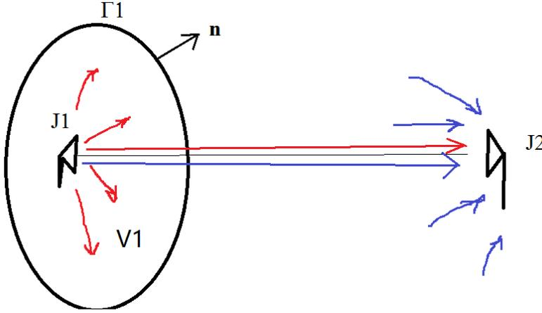
Figure 2., Red arrow is retarded wave, blue line is advanced wave. The arrow direction shows the direction of the energy current. The emitter contains inside the volume  $V_1$ .  $\Gamma_1$  is the boundary surface of  $V_1$ . The energy current consist of the retarded wave and the advanced wave.
