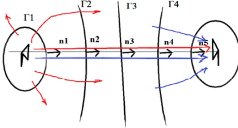
Figure 5: 5 surfaces are shown, the mutual energy current goes through each surface. The integrals of the mutual energy currents with time should be equal to each other in any of the above surface.
