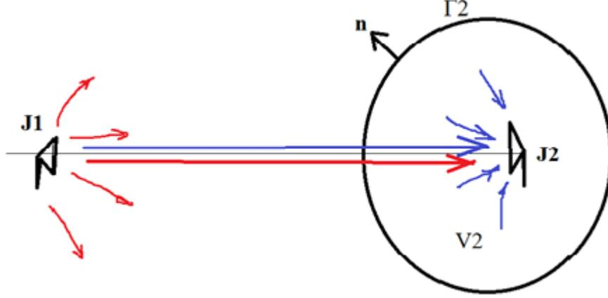
Figure 4: Choose the volume  $V_2$  is close to the absorber. Red arrows are retarded wave, blue arrows are advanced wave. The direction of retarded wave is same as the direction of red arrow. The direction of advanced wave is at the opposite direction of the blue arrow. The arrow direction (red or blue) is always at the energy transfer direction.
