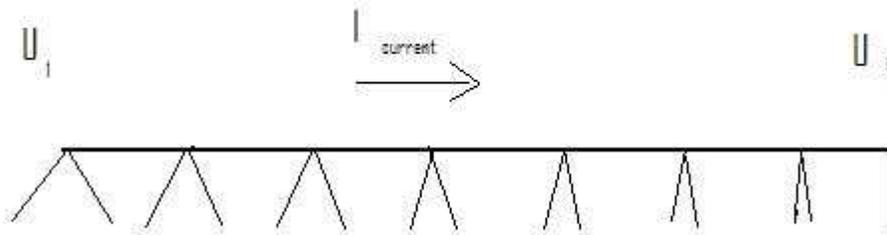
Figure 1.) Aluminium folios shows the charge distribution on the electric wire
