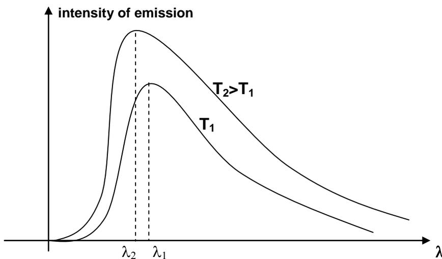
Fig. 3 Emission spectrum of black body for two different temperatures in function of wavelength
