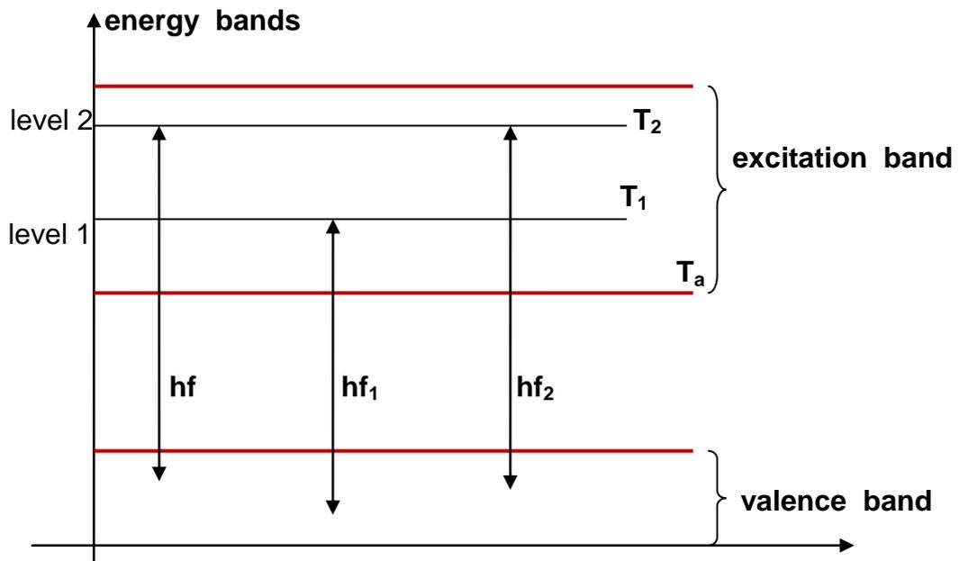
Fig. 2 Energy bands and energy quanta in the condensed matter
