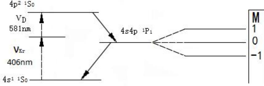
FIG.1. The energy level splitting of the calcium atoms in anomalous Zeeman effect
