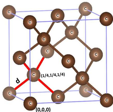
Carbon atoms in diamonds are arranged in a strong tetrahedral structure. The unit cell of a diamond is shown in the figure at left. Here  $a_o$  is the cubic lattice constant and  $d$  is the  $C - C$  bond length of  $0.154nm$ . The four thick lines represent a tetrahedral geometry. The small size of a carbon atom and the tight covalent bond of carbon atoms in diamond structures are responsible for almost all of its unique mechanical, chemical and electronic properties.
