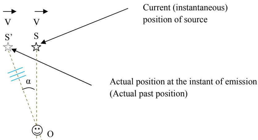
The source position now (at the moment of observation) is at S, moving with velocity V. But the source was at position S' at the moment of emission, moving with velocity V also, assuming uniform motion.
