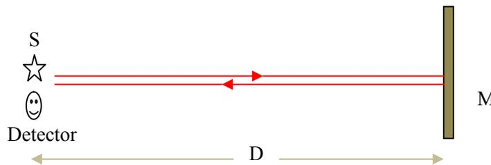
The pulsed light source S and the light detector are very close to each other, so they can be assumed to be at the same point in space. The clock operates as follows. The source S emits a short light pulse, which is reflected from the mirror M back to the detector. Upon detecting the reflected light pulse, the detector actuates the source to emit a light pulse again, which is reflected back to the detector and so on. The rate of such clock is independent of absolute
