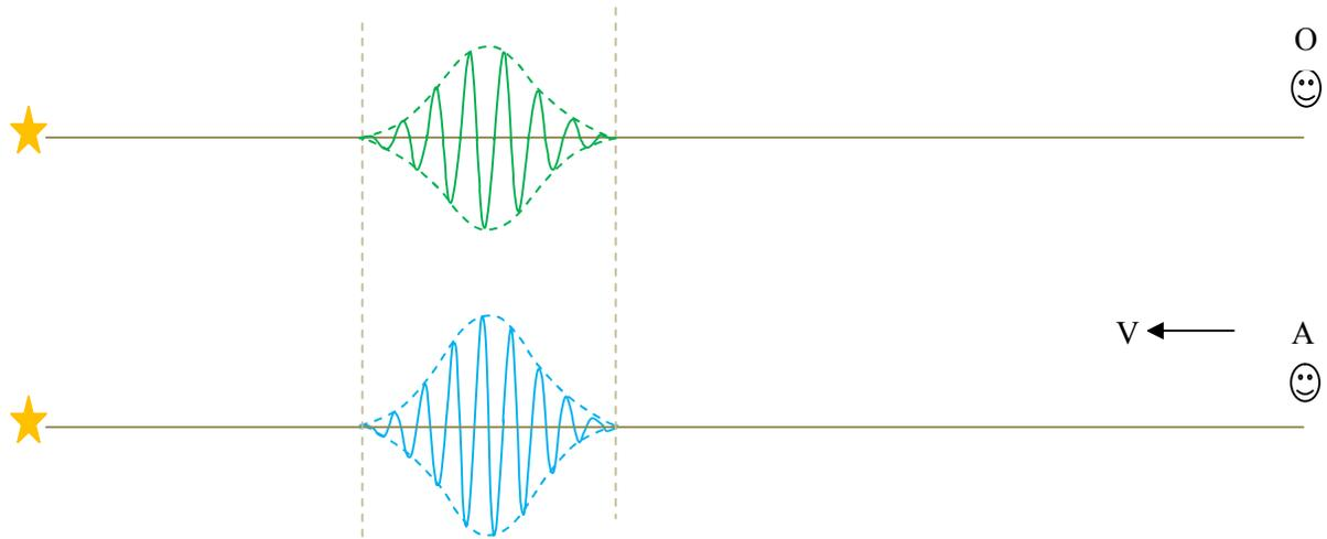
Consider two observers. Observer O is at rest relative to the light source and observer A is moving towards the light source. Suppose that at  $t = 0$ , the source emits a photon and at the same time ( $t = 0$ ), observer A starts moving towards the source with velocity  $V$ .
