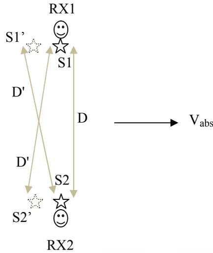
$$\text{Round trip time} = \frac{2D'}{c} = \frac{2D}{\sqrt{c^2 - V_{abs}^2}}$$
