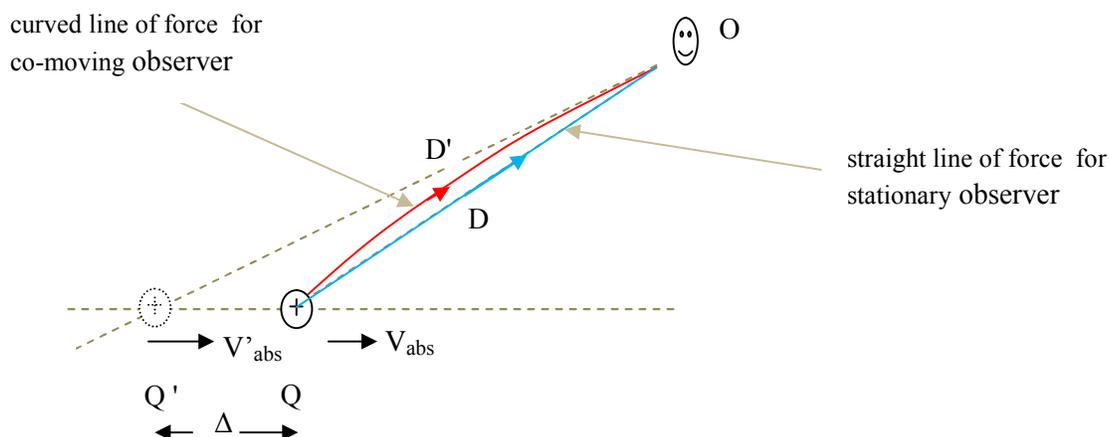
For the stationary observer, it is as if the electric field is rigidly carried by the moving charge, straight radial lines emanating from the charge. We explain this with AST as follows. For the stationary observer, the apparent change in position of the charge is exactly compensated for by the fact that the ‘speed’ of the electrostatic field will be  $c$  relative to the apparent charge  $Q'$ .
