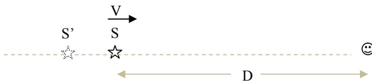
The equations for Doppler effect are the same as above but we see 'aberration' in this case, i.e. the apparent past position ( position of source at the instant of emission ) of source is different from the actual past position.
