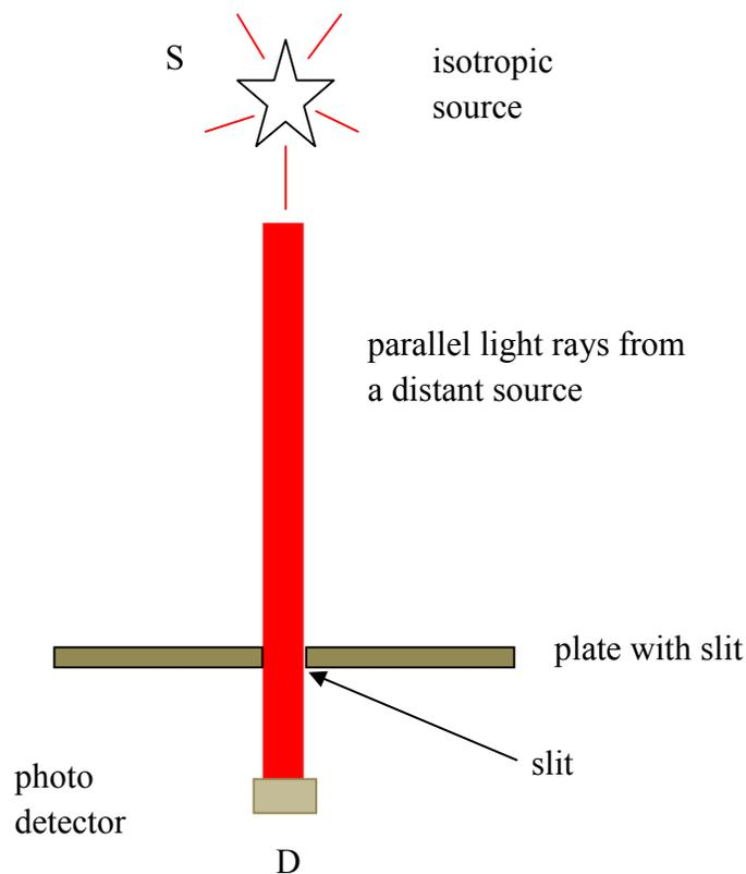
If the whole apparatus is at absolute rest, or if the line connecting the source and the photo detector (line SD) is oriented parallel to the absolute velocity vector, there will be no bending of the light ray.
