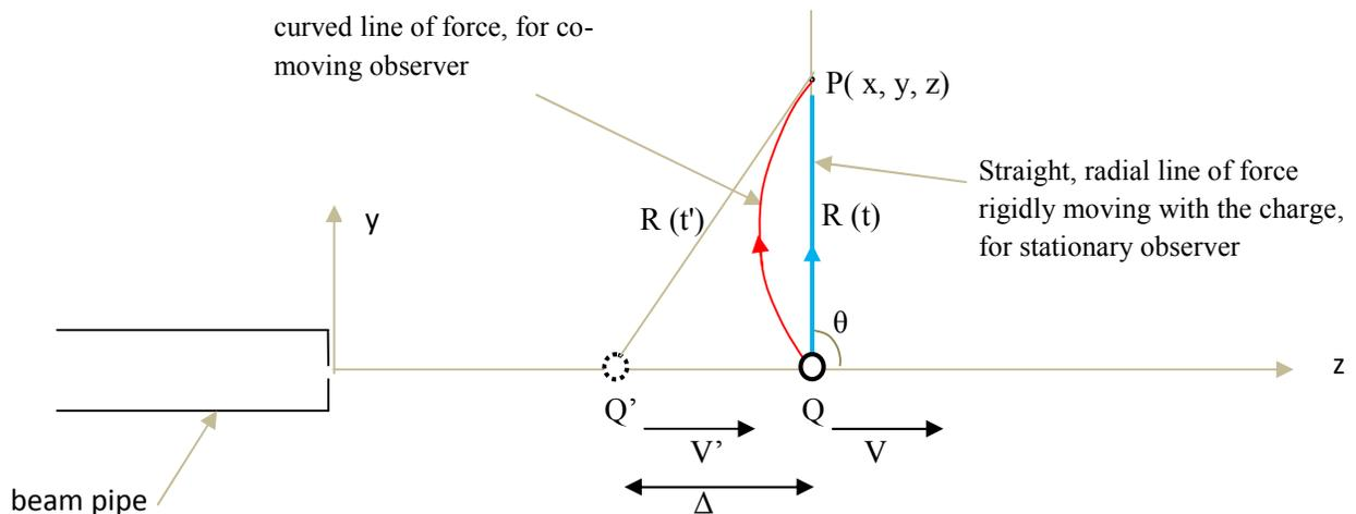
From the figure above, we can see that the maximum transverse electric field is detected at point P when the charge is physically at Q since the detector is at rest.
