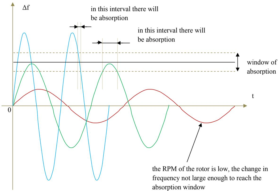
We assumed that there is no absorption at zero angular velocity, because the difference between the resonance frequencies of the source and the absorber is usually made slightly different.
