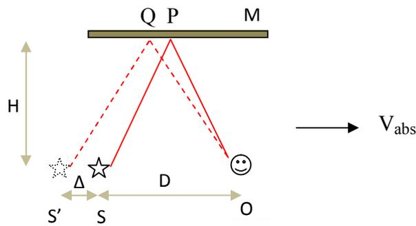
$$\Delta = D \frac{V_{abs}}{c - V_{abs}}$$
