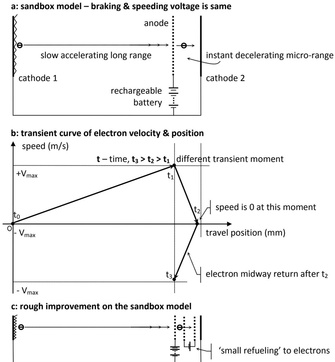
**Fig. 3. tricky braking voltage and short braking distance**
