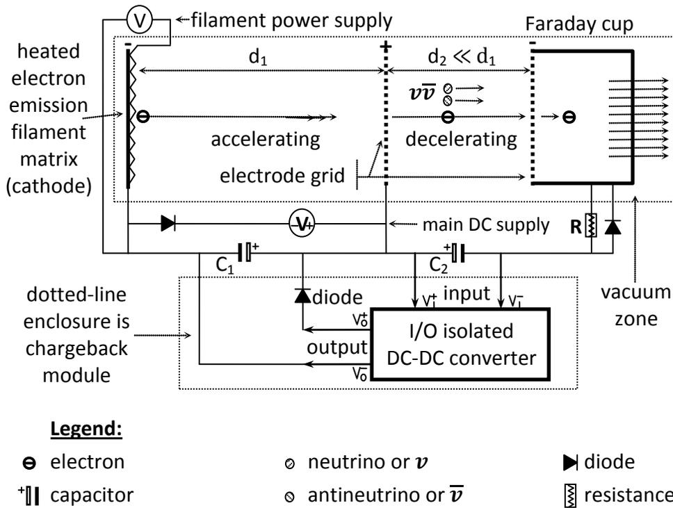
**Fig. 2. Embodiment of artificial low energy neutrinos source**
