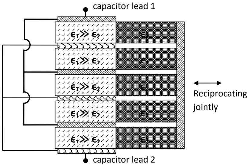
b. parallel mode, total capacitance = embedded\_capacitance\*( $N+1$ )
