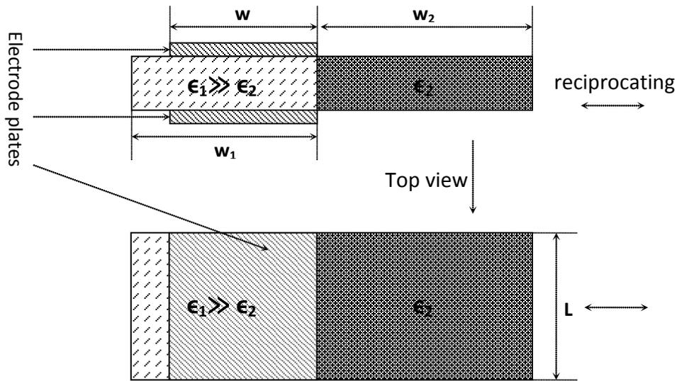
$w_1 > w$  enables excitation voltage enough time to recharge capacitor,
