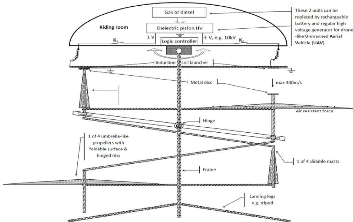
Usually the quartet design creates two quasi air channels where mutual interference may exist, but no significant negative effect, as long as there is proper separation distance between the channels.
