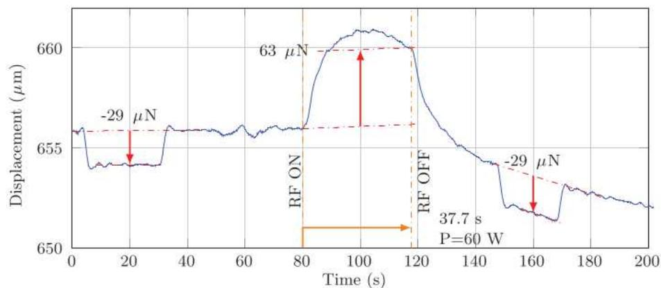
c) 60W forward thrust run at vacuum for split configuration
