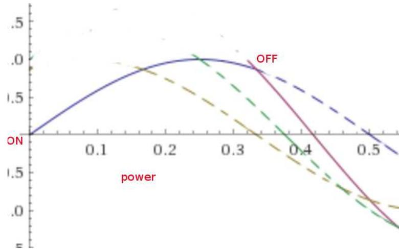
The oscillation is triggered by the "power on" at  $t = 0$ ; the continuous line corresponds to a "power off" occurred shortly after the maximum elongation, as in the previous experimental figure.
