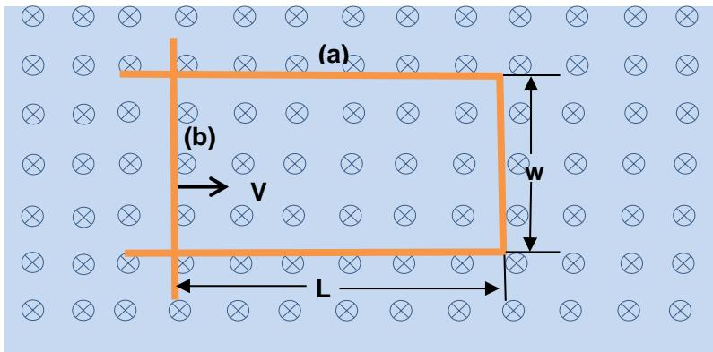
**Fig.1.** A conductor loop consists of two parts, a fixed U shaped frame (a) and a movable crossbar (b) .
