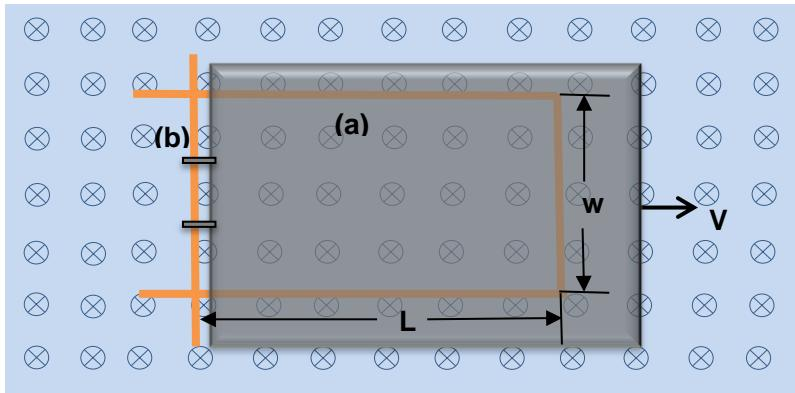
**Fig.2.** The U shaped frame was covered with magnetic shielding material that makes the magnetic field not go through the loop. The others are the same as in figure 1.
