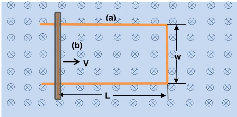
**Fig.3.** The crossbar is covered with magnetic shielding material that makes the magnetic field not reach the crossbar. The others are the same as in figure 1.
