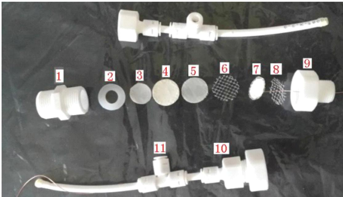
In the figure above, 1 is "A pair of Screw", 2 is the 6 "washer", 3 is " $\phi$ 19mm fine mesh filter", 4 is " $\phi$ 25mmR0 semipermeable membrane", 5 is " $\phi$ 25mm fine mesh filter", 6 is " $\phi$ 25mm diversion mesh", 7 is "surface covered with insulating film, plastic  $\phi$ 19mm copper Foil electrode ", 8 is " $\phi$ 25mm diversion mesh ", 9 is" 6 to 4 tap ", 10 is"
