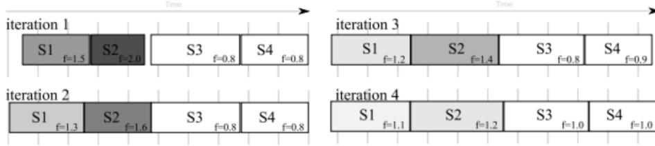
Figure 2: An illustration of the spring based algorithm. Darkness of the colour represents the high speeding up factor. Image taken from the original research paper. [2]
