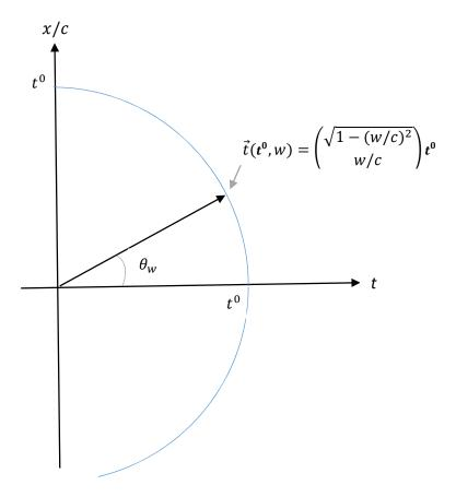
Figure 2 Time vectors,  $\vec{t}(t^0, w) = \binom{\sqrt{1-(w/c)^2}}{w/c} t^0$  for a specific clock time  $t^0$  at an arbitrary position,  $x = wt^0$  on a RF, K; (where  $\sin \theta_w = w/c$ ).
