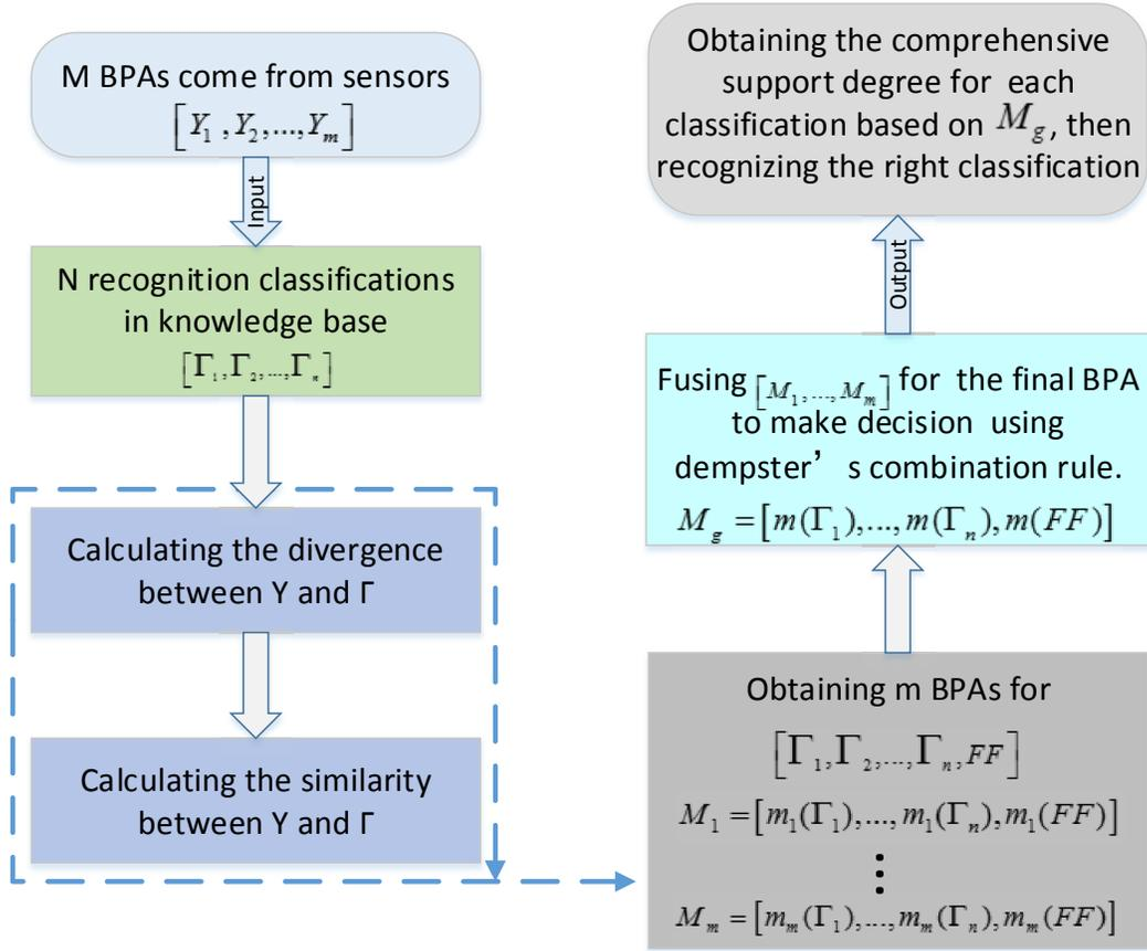
Fig. 4. The flow chart of the proposed algorithm for pattern recognition
