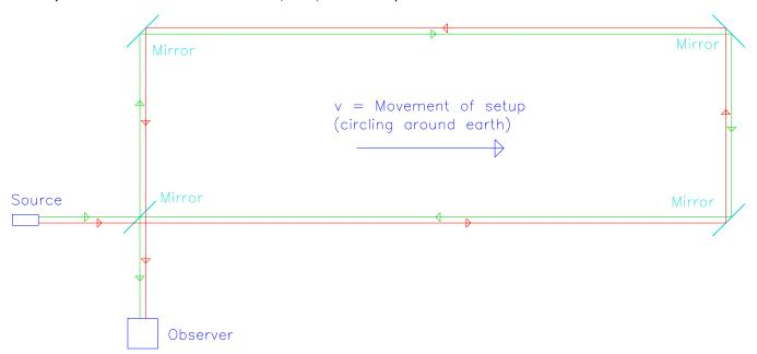
Fig. 7: Schematic setup of the Michelson/Gale/Pearson experiment
