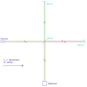
Fig. 1: Schematic setup of the Michelson/Morley experiment
