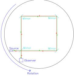
Fig. 4: Schematic setup of the Sagnac experiment
