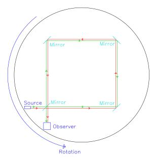
Fig. 12: Schematic setup of the Sagnac experiment
