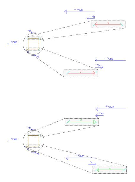
Fig. 13: Velocities on Sagnac experiment in static aether
