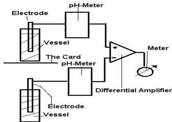
Fig.1 shows a unit diagram of the differential pH-meter.
