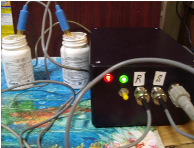
Fig.2. The differential pH-meter with electrodes. R=Reference, S=Sample.
