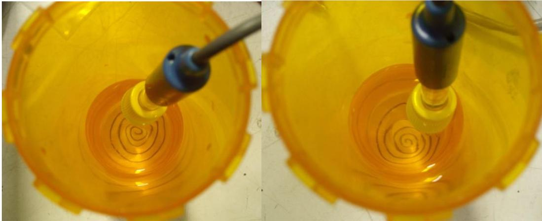
Fig.8. Images of two oppositely twisted spirals are placed under the containers with water and pH-electrodes of the differential pH-meter.
