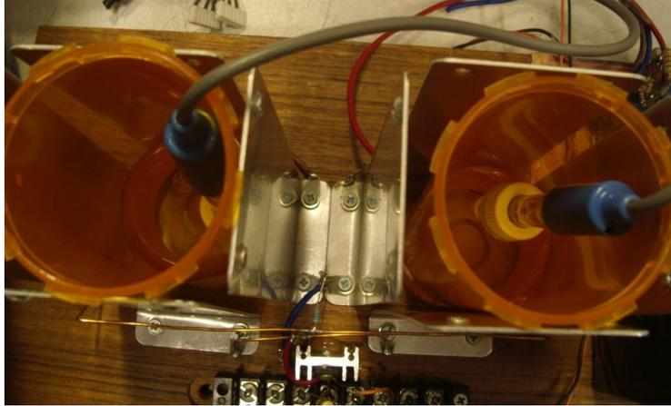
Fig.6. Two identical containers with water and pH-electrodes are placed inside the sources of opposite spinning fields, CCW and CW, 3 MHz, 400 V/m. The electrodes are connected to the differential pH-meter.
