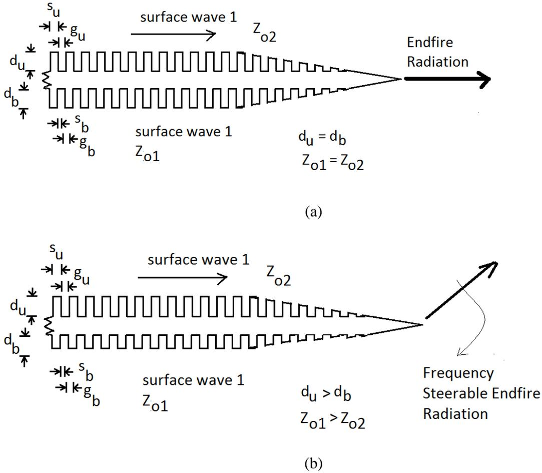
Figure 5. Mechanism of frequency dependent steering of endfire radiation. a) antenna no frequency steerable endfire radiation; b) antenna with frequency steerable endfire radiation.
