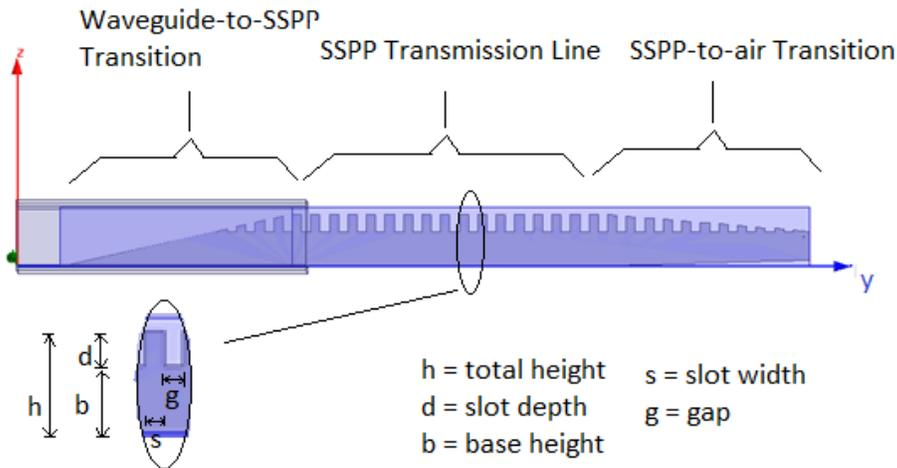
Figure 2. Example of E-plane printed circuit to be mounted in the rectangular waveguide
