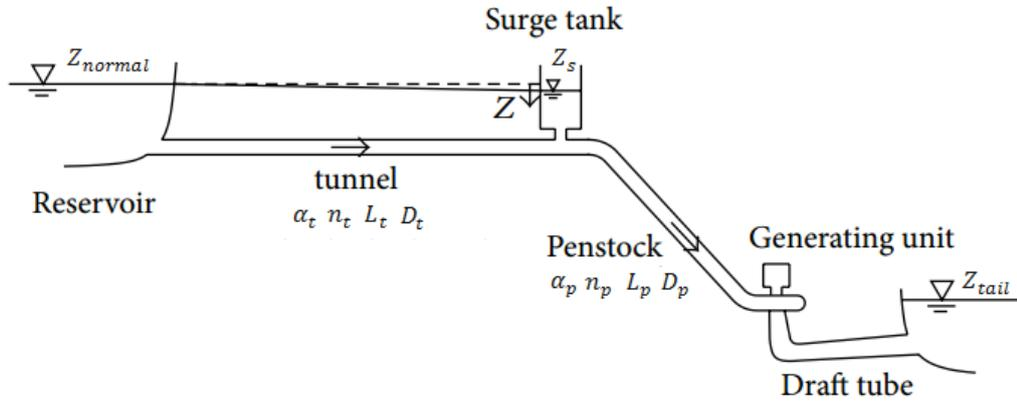
**Figure 1.** Power generating system with surge tank
