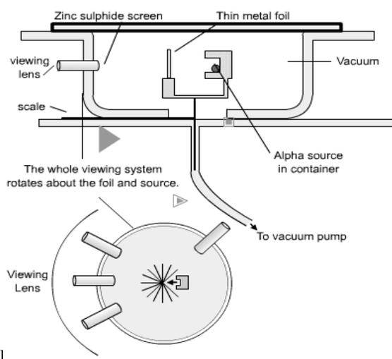
[Fig: Experimental setup for Rutherford's Experiment
