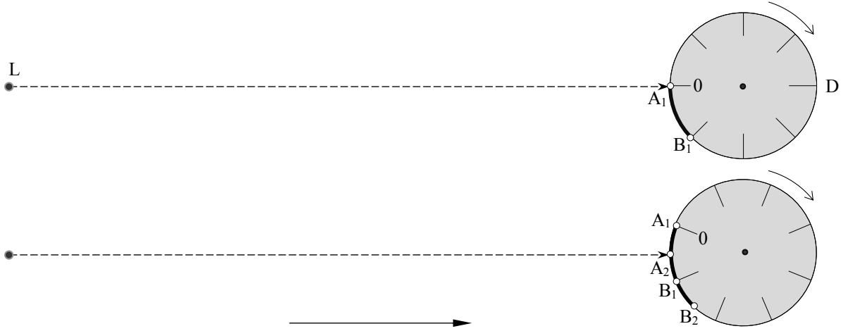
Fig. 4: Schematic of the experimental set-up: A_1 and A_2 denote the points where the rays generated by the first and the second light pulse hit the disk D at the instants t_1 and t_2 . The circular arc length A_1B_1 = d represents the trace on D 's photosensitive lateral surface the very first pulse causes. B_1B_2 = w\delta t_A depicts the trace's length increment produced by the second and any additional pulse according to the propagation hypothesis. The arrow at the bottom indicates the direction of motion of the earth around the sun.
