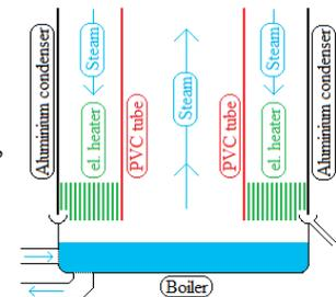
Fig. 6: Installation of the electric air heater.
