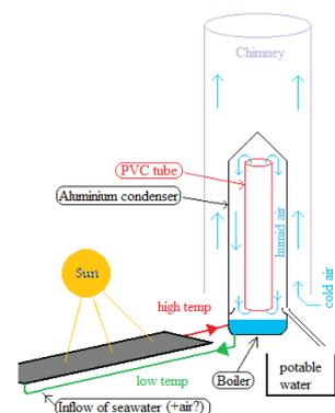
Fig. 3: A solar still with concentric condenser
