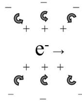
**Fig. 1.** As an electron moves through space nearby quantum dipoles are polarized and rotate.
