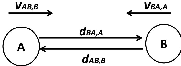
Fig.1 The distance between two inertial observers A and B in relative motion. The velocity  $v_{BA,A}$  is that of observer B as measured by observer A,  $v_{AB,B}$  is that of observer A as measured by observer B;  $d_{BA,A}$  is the distance between A and B measured by A and  $d_{AB,B}$  the distance between A and B measured by B.
