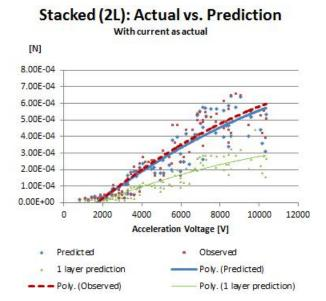
Figure 14: Force versus voltage for double layer capacitor
