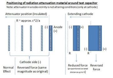
Figure 16: Strategic positioning of radiation attenuation materials
