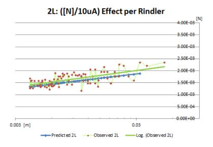
Figure 12: Force versus Rindler distance at  $10\mu A$
