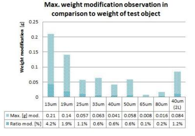
Figure 15: Maximum weight modification for all capacitors
