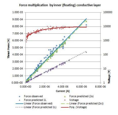
Figure 13: Force versus current for double layer capacitor
