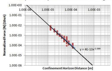
Figure 25: Normalized force versus confinement length
