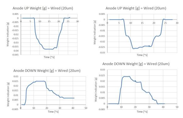
Figure 27: Time Graphs for Wired Setup 2021
