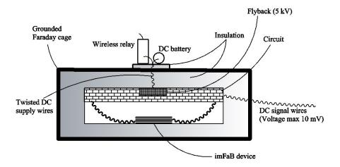
Figure 5: Thruster device
