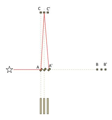
Light from the source hits the beam splitter at point A.The standard analysis starts from the assumption that the transverse light beam will not miss the detector. With this assumption, in the time interval that the beam splitter moves from A to A', the transverse light beam will make round trip time, to meet the beam splitter at point A'. According to the conventional analysis, the longitudinal beam will also go horizontally and exactly reflect back on itself.
