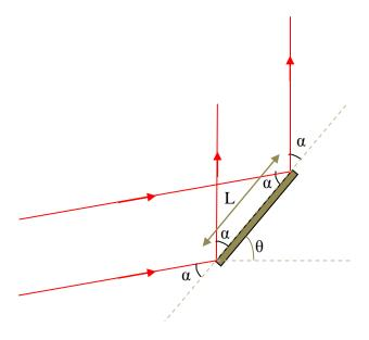
We will consider a simpler case shown below, for a horizontal light ray (angle  $\alpha$  equals angle  $\theta$ ).
