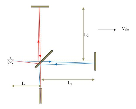
However, I guess that the change in path lengths of the two light beams will depend in a complicated way not only on L1 and L2, but also on L.
