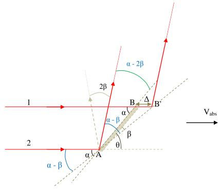
Therefore, the effective angle of incidence is  $\alpha$ -  $\beta$ . The angle of reflection should also be  $\alpha$ -  $\beta$ . Relative to the actual mirror( in the reference frame of the mirror), the angle of incidence is  $90^0$ -  $\alpha$  and the angle of reflection is  $90^0$ -  $(\alpha$  -  $2\beta)$ ! The reflected light ray will be inclined forward by angle  $2\beta$  relative to the reflected ray in the case of zero absolute velocity.
