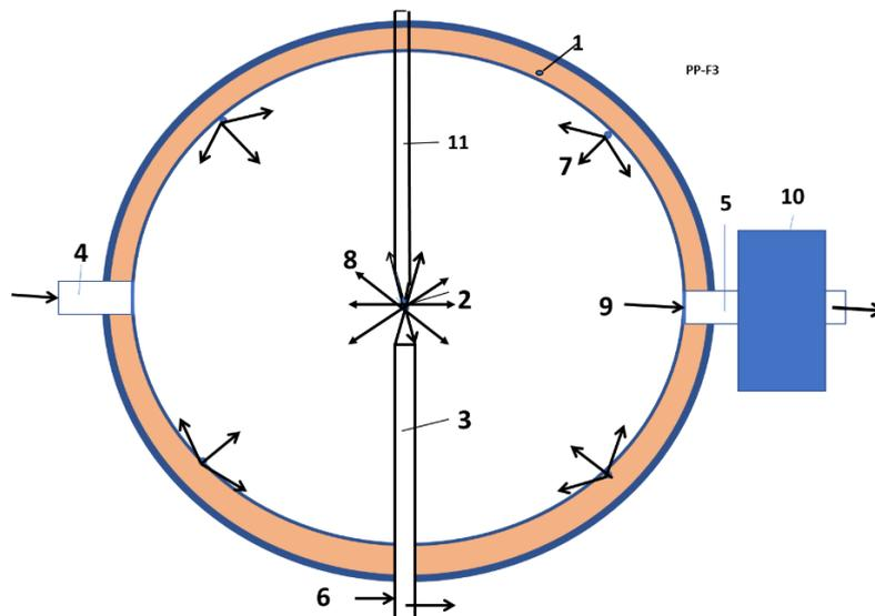
**Fig.3.** Final (industrial) work of Impulse Electric AB thermonuclear reactors. Hot compressed gas from sphere runs to the magneto-hydrodynamic generator (MHG) 10 and produces electric energy or runs to gas turbine and produces an useful mechanical energy.
