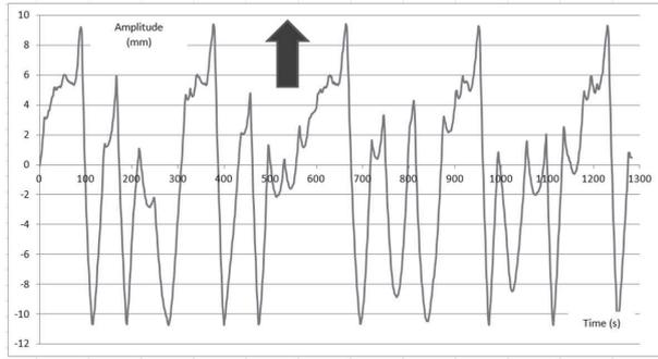
FIG. 3: A part of gravity measure with resonance method. The pendulum movement in "plan view". The black arrow shows the direction of the source masses.
