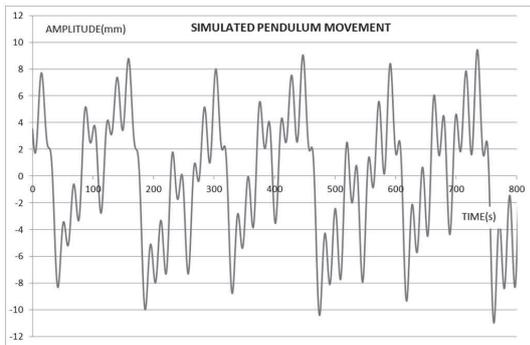
FIG. 4: The simulation of the dynamic gravity measure corresponding to FIG. 3. The calculated pendulum movement vs. time.
