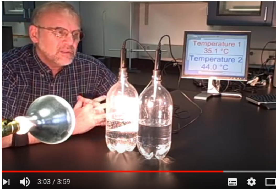
Figure 56. Greenhouse Gas Bottle Demonstration [92]. Bottles with CO 2 and air are radiated and temperature measured – CO 2 in blue. Is this not an experiment to measure the heat capacities of the respective gases?
