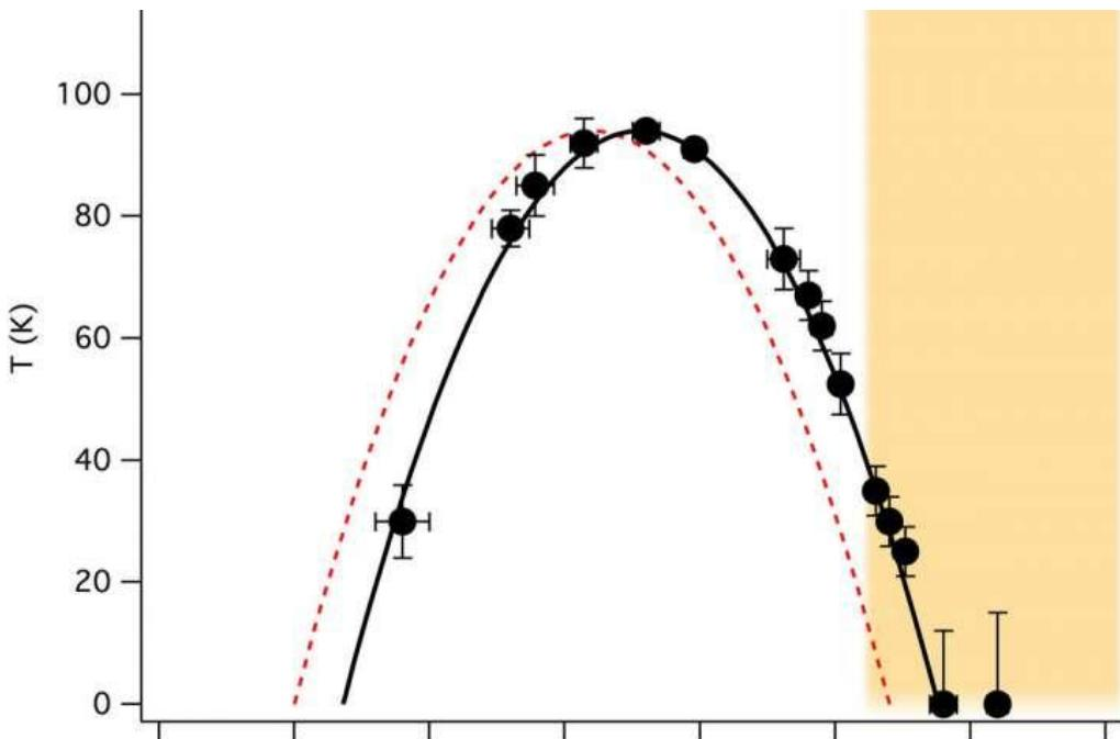
This phase diagram for BSCCO plots the temperature ( $T$ , in degrees Kelvin, on the y axis) at which superconductivity sets in as more and more charge vacancies, or "holes," are doped into the material (horizontal, x axis). On the underdoped ...more"Until this study, nothing past that point was known because we couldn't get crystals doped above that level. But our new data takes us to a point of doping way beyond the previous limit, to a point where  $T_c$  is not measurable."
