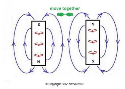
Figure 9b: Permanent magnets: side-by-side: opposite rotation/spin: move together.
