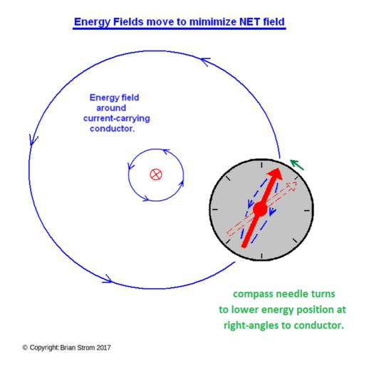
Figure 8b: Interaction between compass needle and current-carrying conductor.
