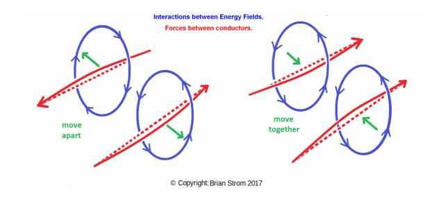
Figure 7: Interaction between Energy Fields around conductors.
