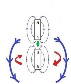
Rotating energy field subtracts from the magnet's field: floating magnet moves downward.
