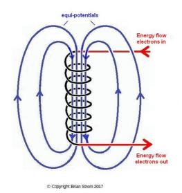
Potential Energy Field around coiled conductor
