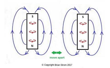
Figure 9a: Permanent magnets: side-by-side: same rotation/spin: move apart.
