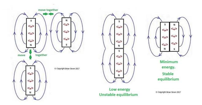
Figure 15: Minimum energy configurations for energy fields.
