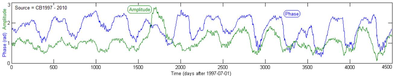
The further investigations are carried out with the method of direct conversion: To measure the phase constancy and the amplitude of the signal, this is multiplied by a computer-generated sinusoid of the same frequency.
