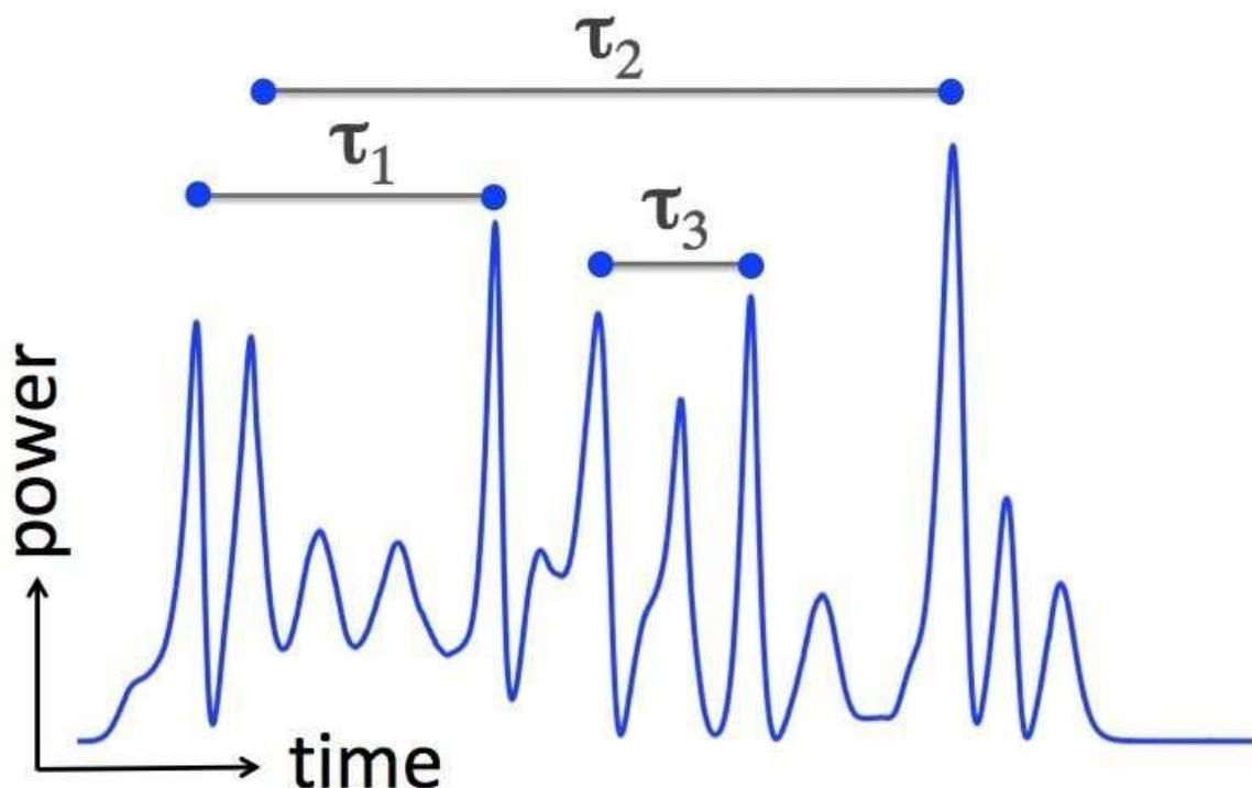
Simulated profile of an X-ray pulse from an X-ray free-electron laser. It consists of a train of narrow spikes whose intensities (power) fluctuate randomly. SLAC researchers suggest using pairs of these spikes for pump-probe experiments that trigger and measure structural changes in a sample, turning a former nuisance into an advantage. This example highlights three pairs of spikes with different time delays between them. Credit: SLAC National Accelerator Laboratory
