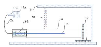
Figure 14: 800W 5.8 GHz magnetron AIR-COOLED (1a), Universal magnetron launcher and WR159 transition waveguide to N-type female connector (UML-TW) (1b.), 1m coaxial cable with N-type male connector to N-type female bulkhead (2a.), internal aerial system (3-6.), 74MM ID 1130MM long aluminum cavity tube (9a.), Aluminum tube suspended horizontally from swivel-arm (11.) by spring (10.), measurement rulers to measure movement at the distal end (12.), anticipated direction of thrust/movement (14.)
