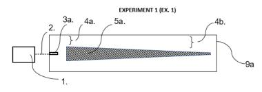
**Figure 3: EX-1**; AC/pulsing power supply for solenoids (1.), connecting coaxial lead (2.), chamber coupling pin (3a.), chamber ideal circumferential distance 25.8mm (4a.), chamber non-ideal circumferential distance ~31mm (4b.), internal steel rod tapered from 22.3mm diameter to 12mm diameter (5a.), aluminium tube cavity chamber 74mm ID (9a.).
