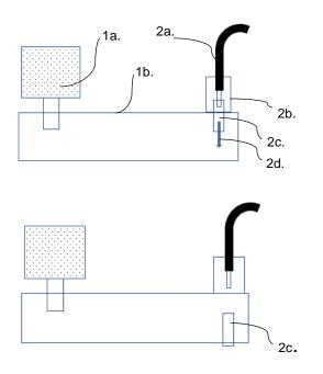
**Figure 8: EX-1**; 800W 5.8 GHz magnetron AIR-COOLED (1a), Universal magnetron launcher and WR159 transition waveguide to N-type female connector (UML-TW) (1b.), 2m coaxial cable with N-type male connector to N-type female bulkhead (2a.), N-type female bulkhead (2b.), coupling pin (2c.), direction of thrust of coupling pin (2d.)
