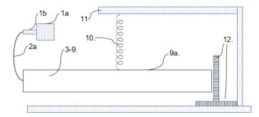
**Figure 5**: 800W 5.8 GHz magnetron AIR-COOLED (1a), Universal magnetron launcher and WR159 transition waveguide to N-type female connector (UML-TW) (1b.), 1m-2m coaxial cable with N-type male connector to N-type female bulkhead (2a.), internal aerial system (3-9.), 74MM ID 1130MM long aluminum cavity tube (9a.), Aluminum tube suspended horizontally from swivel-arm (11.) by spring (10.), measurement rulers to measure movement at the distal end of resonance cavity tube (12.)
