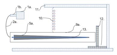
Figure 7: 800W 5.8 GHz magnetron AIR-COOLED (1a), Universal magnetron launcher and WR159 transition waveguide to N-type female connector (UML-TW) (1b.), 2m coaxial cable with N-type male connector to N-type female bulkhead (2a.), internal aerial system (3-9.), 74MM ID 1130MM long aluminum cavity tube (9a.), Aluminum tube suspended horizontally from swivel-arm (11.) by spring (10.), measurement rulers to measure movement at the distal end (12.), blue arrow anticipated direction of movement (13.)
