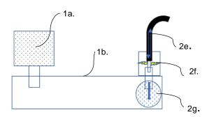
**Figure 10: EX-1**; 800W 5.8 GHz magnetron AIR-COOLED (1a), Universal magnetron launcher and WR159 transition waveguide to N-type female connector (UML-TW) (1b.), proposed resonance field effect in coaxial cable (2e.), proposed arcing in female bulkhead cavity (2f.), proposed region of EM resonance field in magnetron launcher (2g.)
