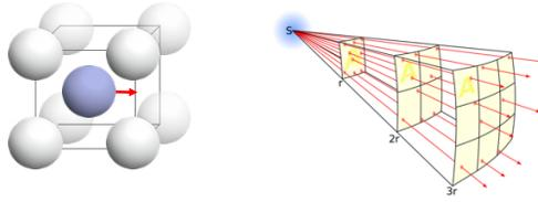
**Fig. 1 – Body centered cubic unit cell (left) and inverse square relationship (right)**
