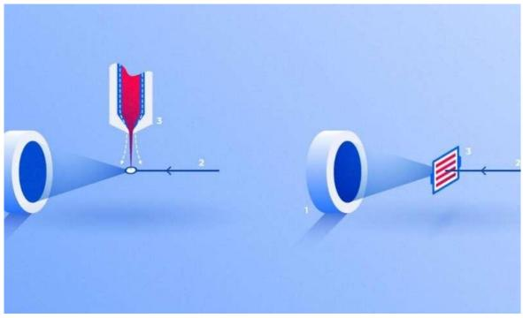
Two ways for feeding crystals into the operating area of the device: in a stream of liquid (3, left) and on a solid substrate (3, right). In both cases, the X-ray beam (2) passing through crystals generates a diffraction pattern on the screen (1). Credit: Elena Khavina/MIPT
