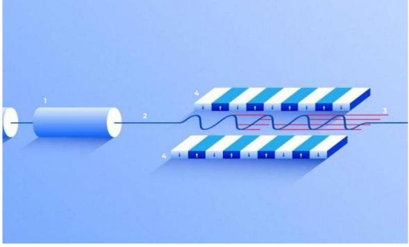
X-ray free-electron laser. A source (1) emits free electrons (2) moving merely tens of times slower than the speed of light through the undulator (4), a tunnel lined with many magnets. The magnetic field causes an electron traveling through the tunnel to oscillate and therefore emit X-rays. The movement of the electrons in the undulator is synchronized to generate tight, high-frequency X-ray pulses of remarkable intensity (3). Credit: Elena Khavina/MIPT
