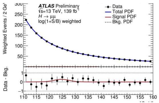
This new ATLAS result shows a search for the Higgs boson decaying to a pair of muons. The measured muon pair mass distribution is shown, combined over all categories. Credit: ATLAS Collaboration/CERN
