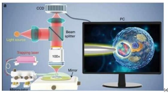
Schematic illustration of the experimental setup. A conventional reflection-mode microscope equipped with a CCD camera and ×100 objective lens was used to observe samples and record images. The inset shown in a PC screen schematically depicting how the biomagnifier is used to magnify and image the subcellular structures inside a bio sample. Credit: Light: Science & Applications, doi: 10.1038/s41377-019-0168-4
