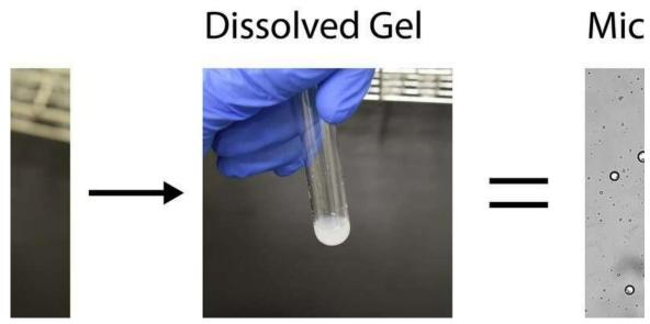
Alpha-hydroxy acid monomers are dried, resulting in the synthesis of a polyester gel. This gel is then rehydrated, resulting in the assembly of microdroplets. Credit: ELSI
