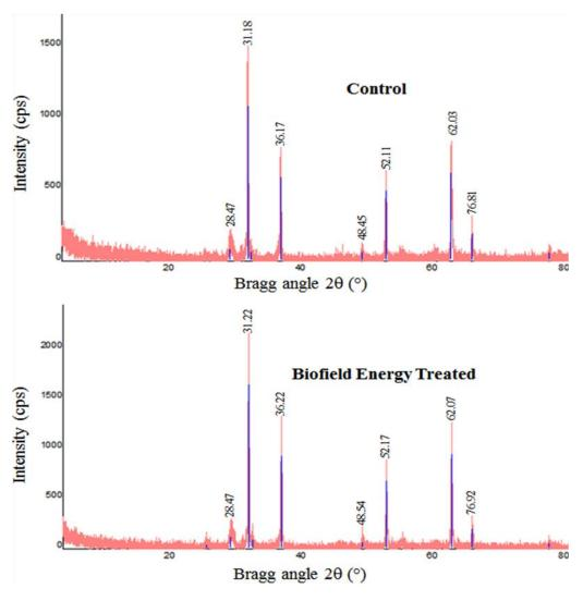
Figure 1: PXRD diffractograms of the control and Biofield Energy Treated lead.
