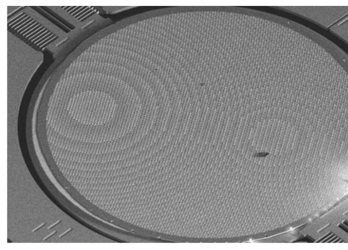
In this image, a circular metasurface-based flat lens has been integrated onto a MEMS scanner. Integration of MEMS devices with metalenses combine the strength of high-speed dynamic control with precise spatial manipulation of wave-fronts. ...<u>more</u>
