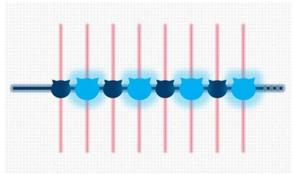
Sketch of the experiment: Rubidium atoms are captured by laser beams (red). Another additional laser (blue) excites about half of the atoms to such an extent that their atomic shells merge with the adjacent atoms. Credit: Forschungszentrum Jülich/Tobias Schlößer
